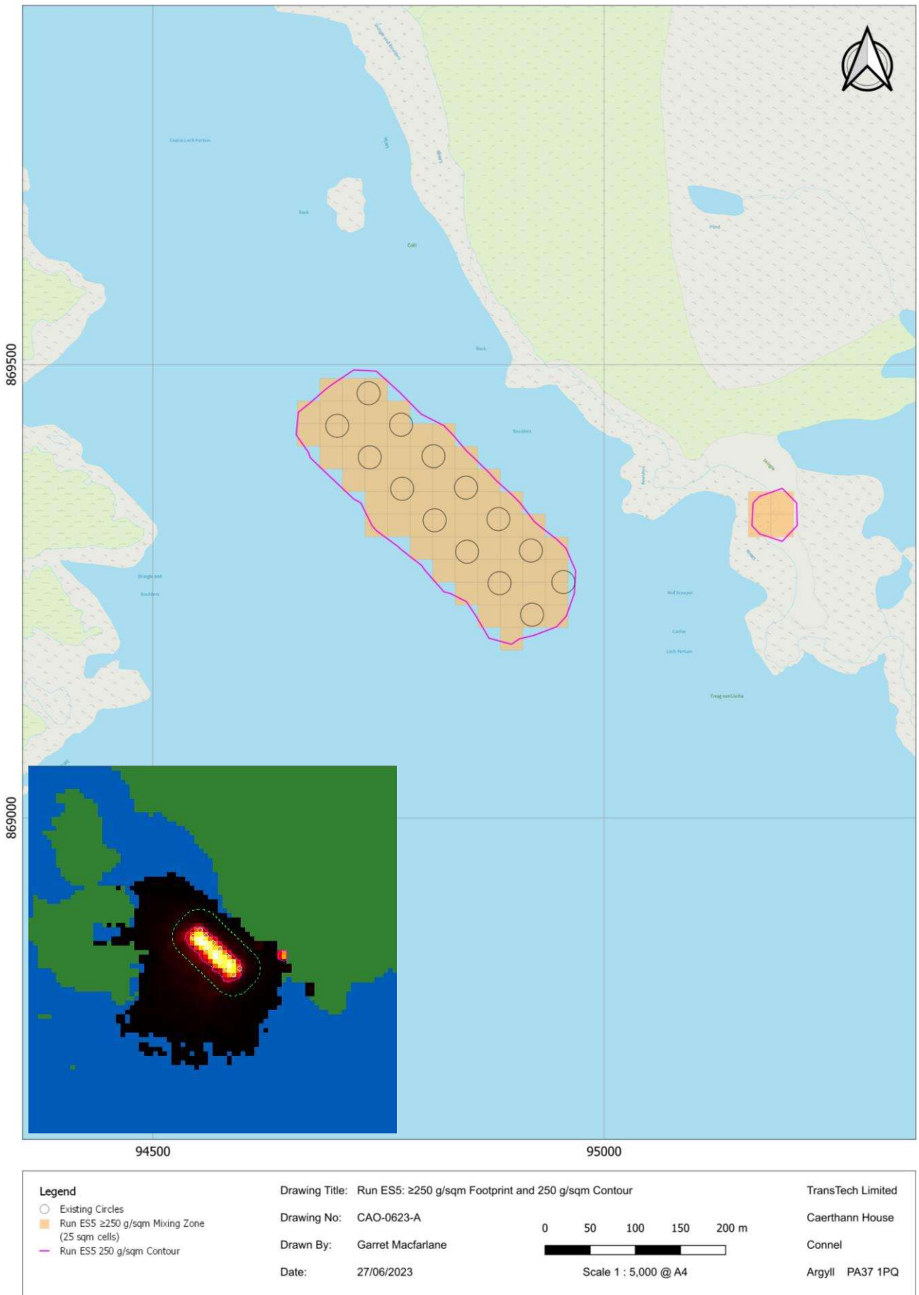
Figure 4. Run ES5 (average for days 275-365): 44,375 m 2 mixing zone area and 250 g/m 2 contour. UI plot also shown.
