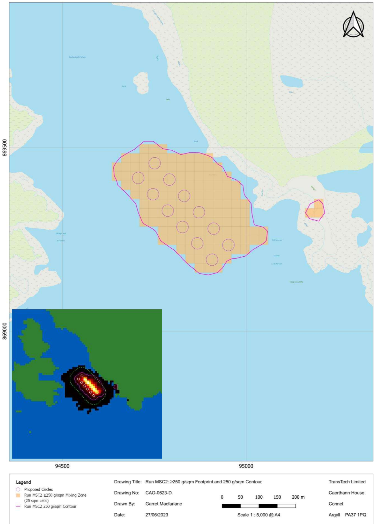
Figure 8. Run MSC2 (average for days 275-365): 250 g/m 2 modelled footprint and this run's 88,750 m 2 mixing zone area along with the UI's display of this.
