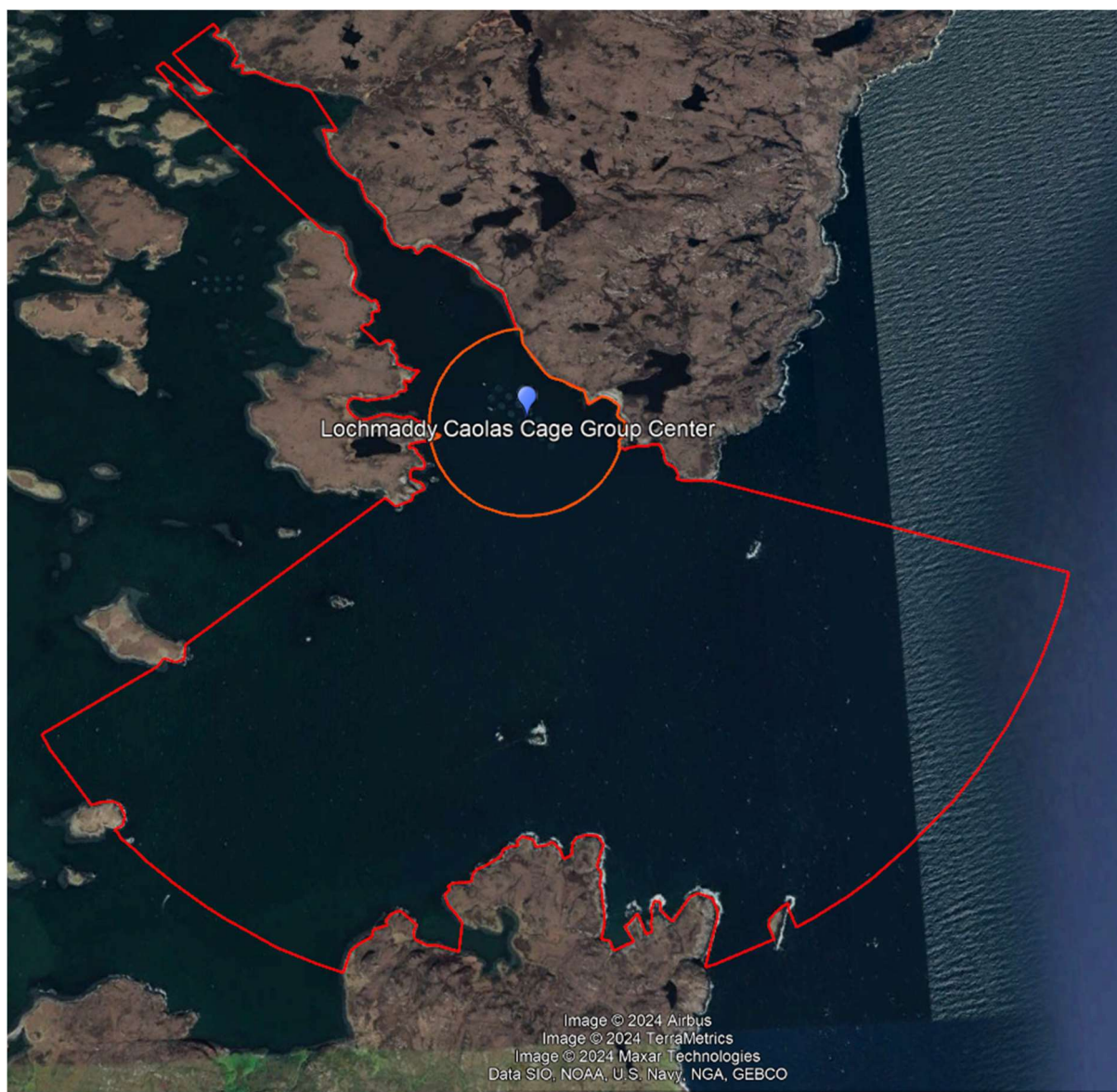
Figure A3 Sea area that lies within the disturbance threshold radius (2,154m from the site centre; red line). The orange line represents the sea area within the PTS threshold radius (379m) for cetacean species with very high frequency hearing range (i.e. harbour porpoise). The PTS threshold for cetaceans with high frequency (dolphins) and low frequency (whales) hearing ranges are 24m and 25m respectively and are not shown on the figure. Blue marker = proposed site centre.
