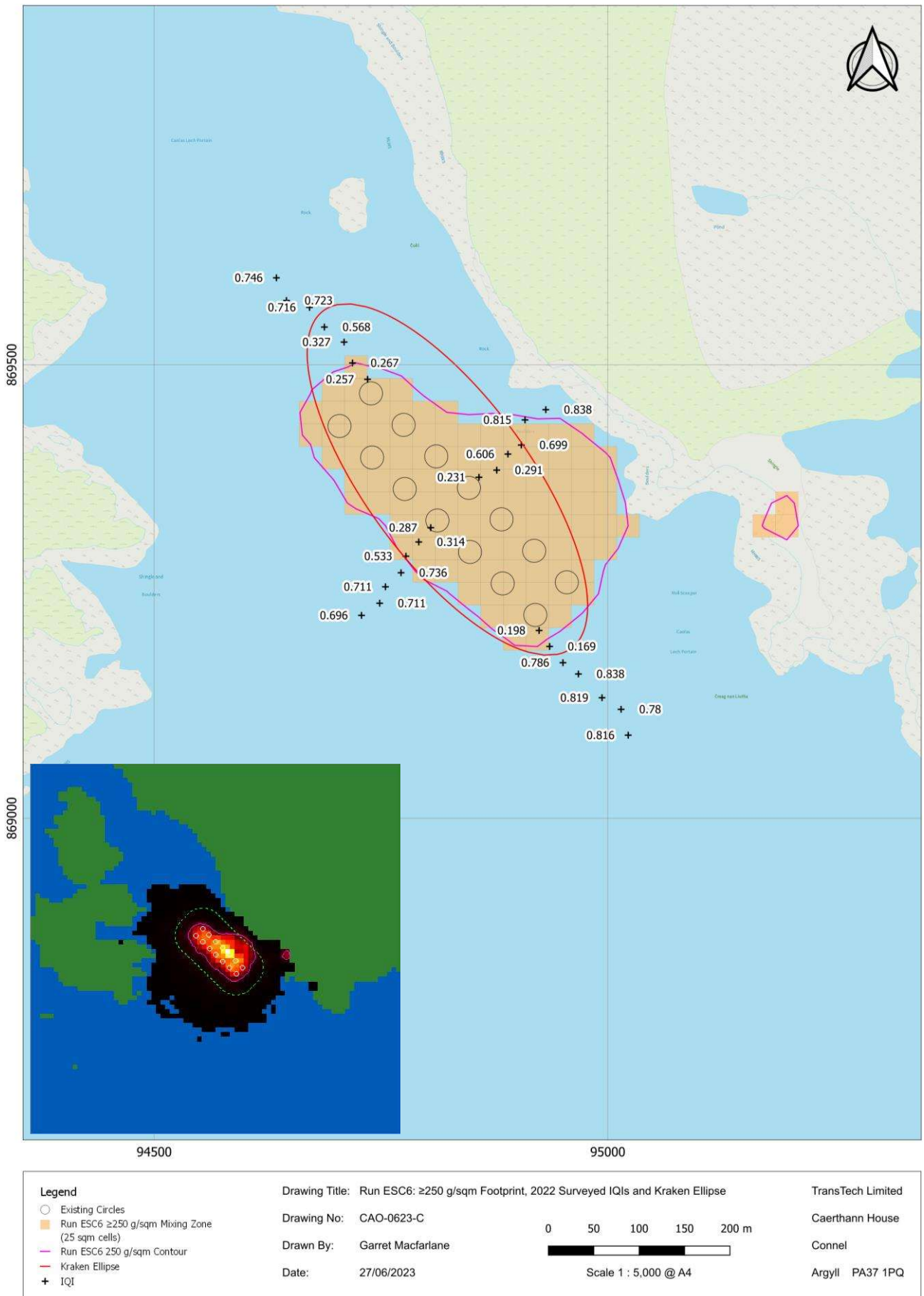
Figure 7. Run ESC6 (average for days 275-365): 66,250 m 2 mixing zone area, 250 g/m 2 contour, 2022 benthic survey IQIs and 0.64 IQI ellipse from Kraken (NB: this is the RStudio plotted ellipse (area = 64,416 m 2 ) which is slightly larger than the 5 th percentile area of 64,416 m 2 ). UI plot also shown.
