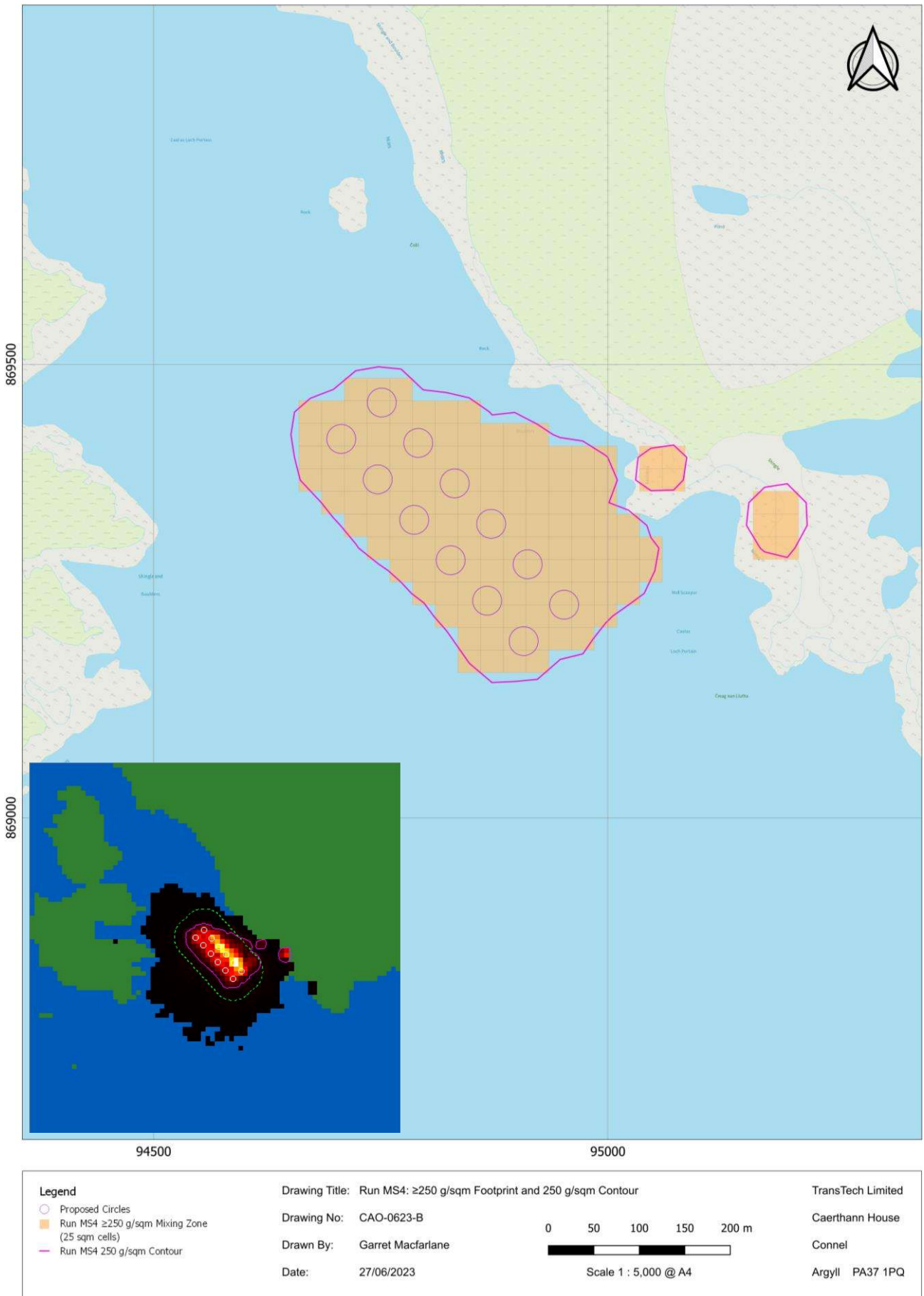
Figure 5. Run MS4 (average for days 275-365): 86,875 m 2 mixing zone area and 250 g/m 2 contour. UI plot also shown.
