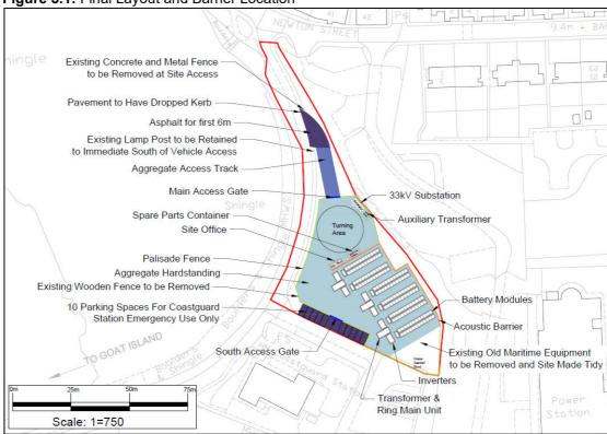
5.3 The acoustic barrier should be continuous with no gaps, either between sections or at the base or sides of the barrier. The mass of a barrier should be at least 10kg/m<sup>2</sup>. As 19mm thick softwood boards have a mass of approximately 10.5kg/m2 they would be suitable for the proposed barrier as long as it was suitably maintained. The barrier could also be constructed of brickwork. The location of the barriers can be seen in Appendix C.
