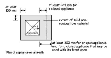
The 150 mm does not apply where the appliance is located in a fireplace recess, nor does it apply where the back or sides of the hearth either abut or are carried into a solid, non-combustible wall.
