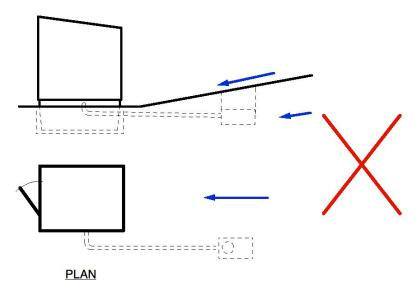
Ground water around the soakaway could cause vaults to flood!!
