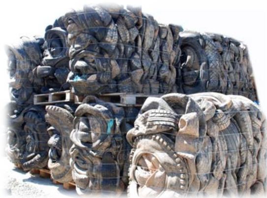
Figure 4 Baled tyres ready for engineering work
