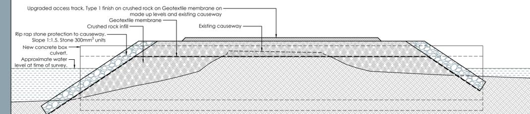
Causeway upgrading - Section to east of box culvert
