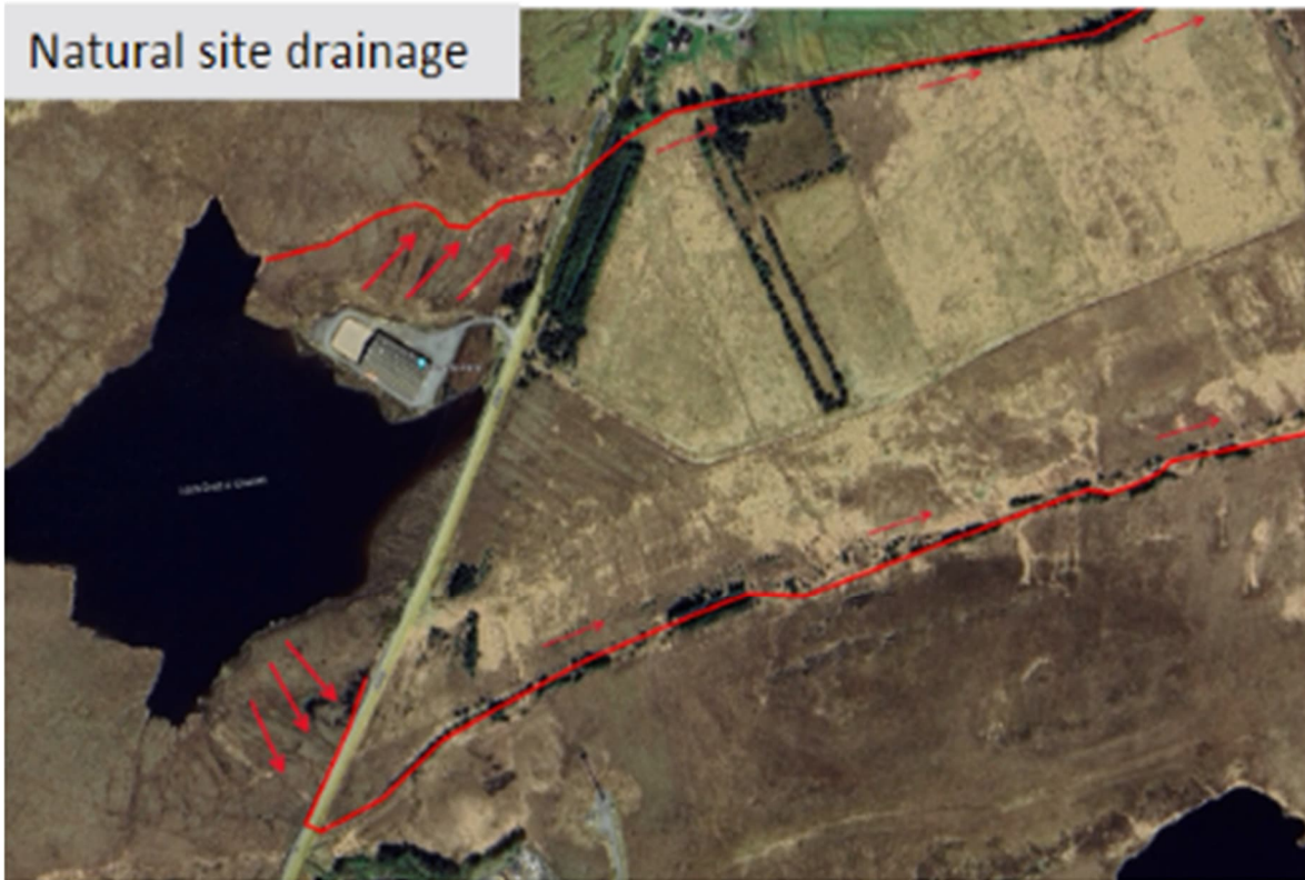
Figure 2-2: Existing Drainage of Arnish Moor Site
