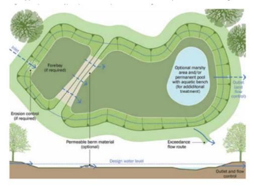
Figure 4-4 Typical detail of a detention basin with a forebay or settlement lagoon.
